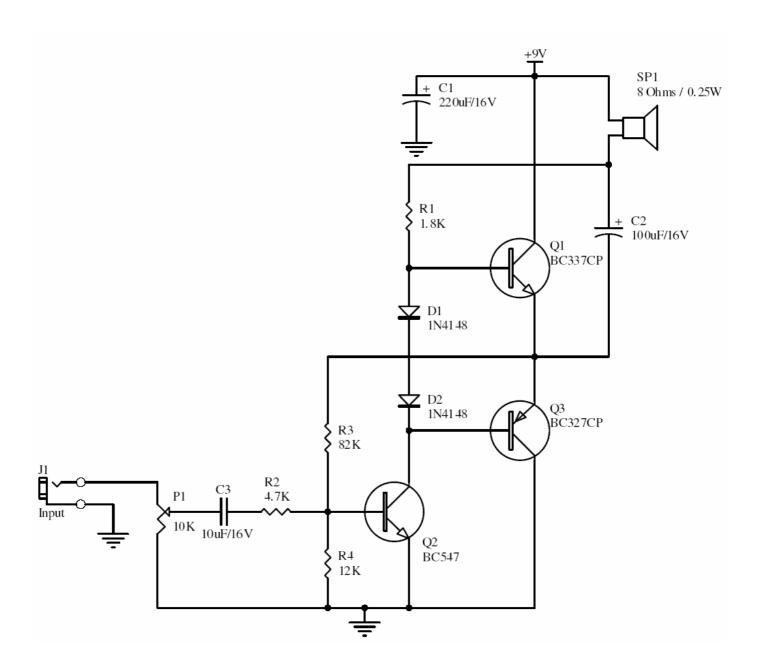
This is a low watt audio amplifier with a different technique in design. The 1.8K resistor has been connected to output of the circuit instead of VCC line. The output power of the circuit is about 250mW on an 8 ohms small speaker.
